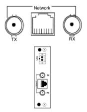
Figure 4. K Module Rear Panels, Showing Location of Connectors
